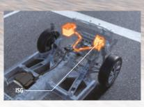
RESTART Press the accelerator and the ISG functions as a starter motor to silently and smoothly restart the engine
