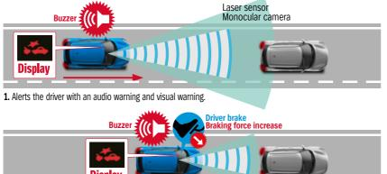
2. Deploys brake assist to increase braking force if the risk of collision is high and the driver panic brakes.
